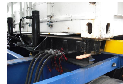
On board hydraulic rams to lift container free of trailer to change configuration
