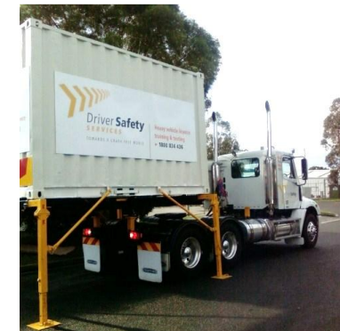
Installing container on prime mover for Heavy Rigid configuration
